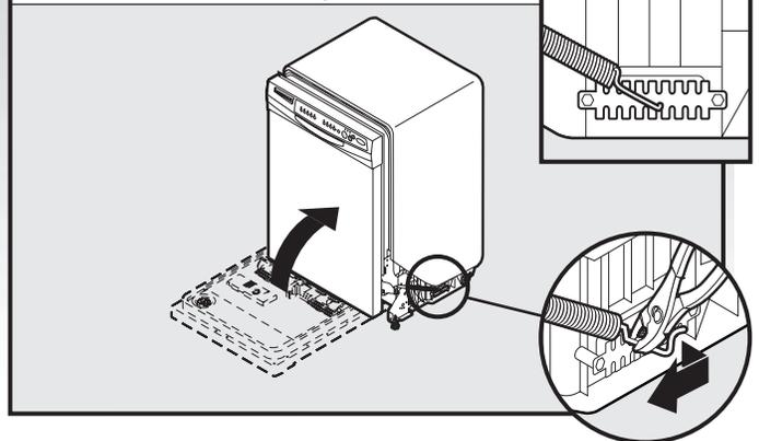
If the door closes too quickly, decrease the spring tension by moving the spring end toward the front of the dishwasher.
